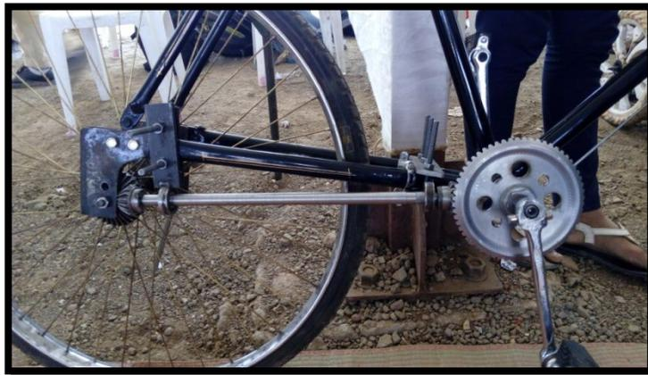
*Fig.1: Shaft driven bicycle*
